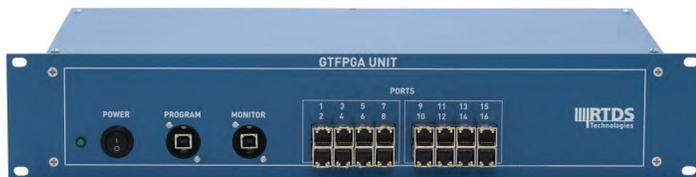
The GTFPGA-SV component provides IEC 61850-9-2LE and IEC 61869-9 Sampled Values (SV) communications using the GTFPGA Unit hardware. The use of dedicated FPGA-based hardware significantly increases the number of SV data streams that can be output from the RTDS Simulator.
